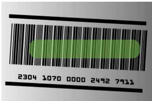
The green light bar should be approximately centered on the bar code and cover approximately 3/4 of a wide bar code
